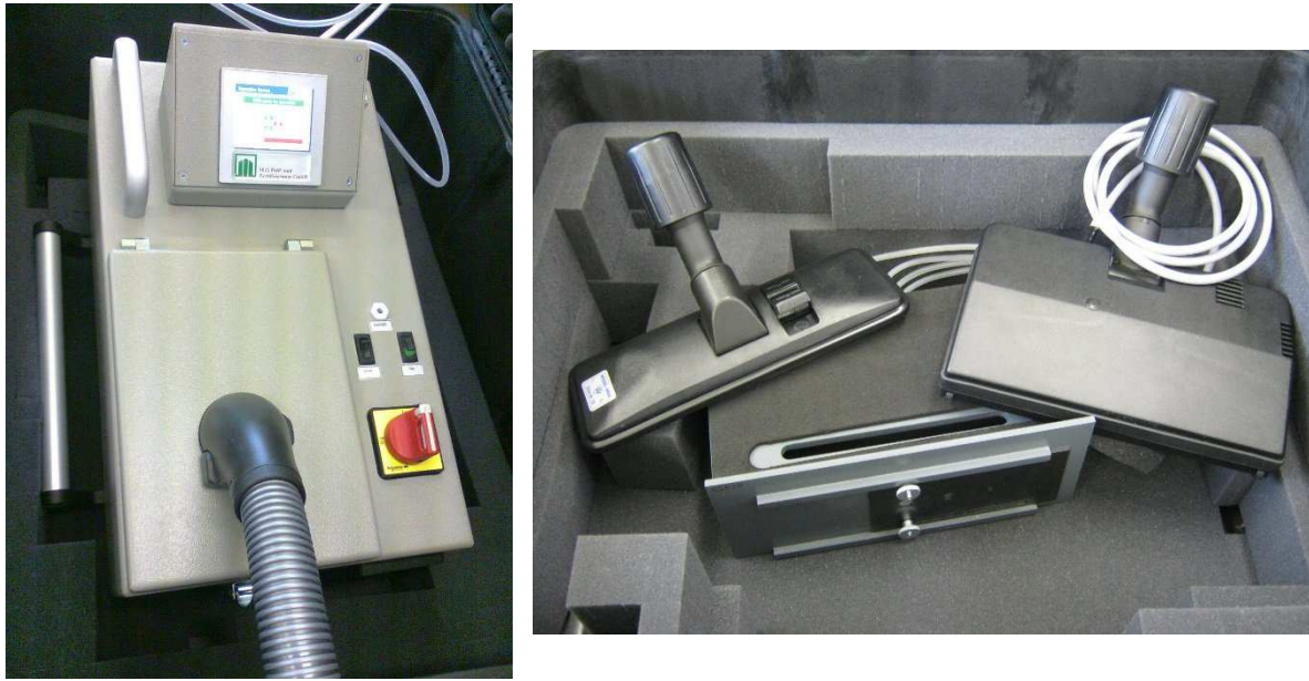
Figure D.1 – RSB with passive and active nozzle and vacuum calibration test box
